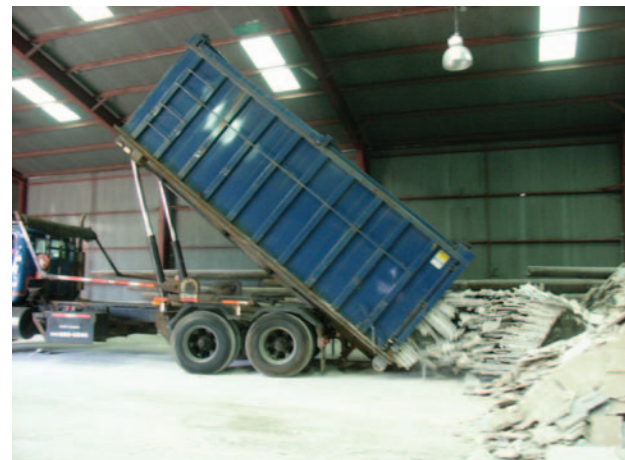
Below: Delivery of new construction waste plasterboard by container truck at GRI's Boston facility.
