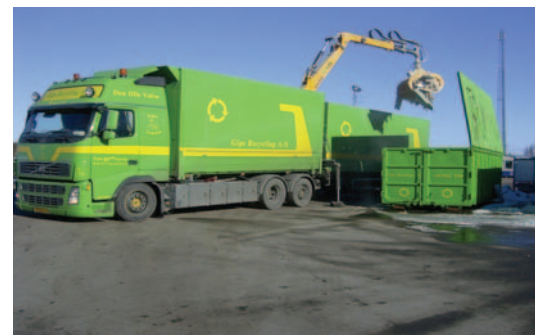
Above: Special grab trucks collect the plasterboard waste from the containers thereby saving transport costs.
