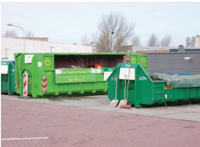
Above: Dedicated plasterboard recycling container at a public recycling centre, where the public makes the segregation.
