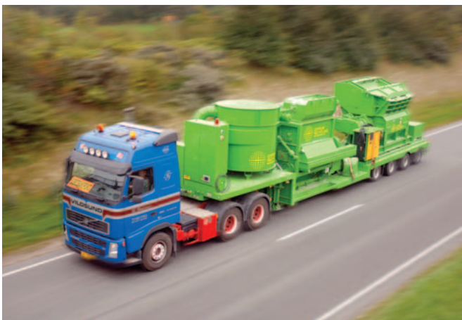
Below: Gypsum Recycling International's XL recycling unit model: the biggest plasterboard recycling unit in the world, but still mobile on two trailers. It can be transported everywhere in Europe and North America. Capacity: 200,000t p.a.
